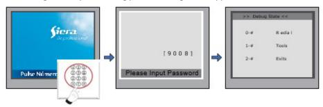
When Door Station is in standby, press '#' key input '9008', then input the Admin Code. (66666666 by default) Debug State menu is launched
