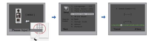
Press "#", Input "8002", then input Setup Code or Admin Code(88888888 or 66666666 by default) Press "4" to enter unlock code item.
