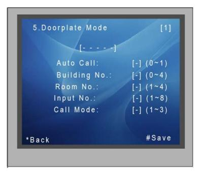
Auto Call: 0 means calling Automatically After press room number 1 means press "#' to call after pressing room number
