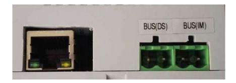
RJ45: Connect to Ethernet Switch or Optical fiber for network
