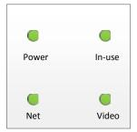
Power: Flashing is in starting, Normally ON means standby status
