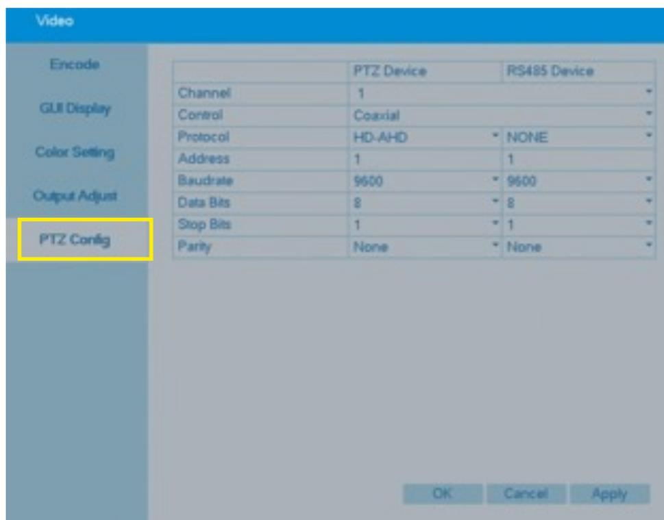
**5. Within this configuration you must configure the communication parameters that you will use with the camera.**
