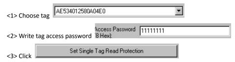
According to EPC number of the tag, setting read protection, make tag unable to be read and written by any order, even if query the tag, it is unable to get EPC number of the tag. Only NXP UCODE EPC G2X tags valid.
