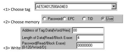
Start address: 0x00 stand in start to read data from first word in the designated storage area, 0x01 stand in start to read data from second word in the designated storage area, and so on.
