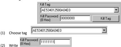
Kill password can not be the whole 0. Otherwise, the tag can not be killed, and the tag return response with parameter error.
