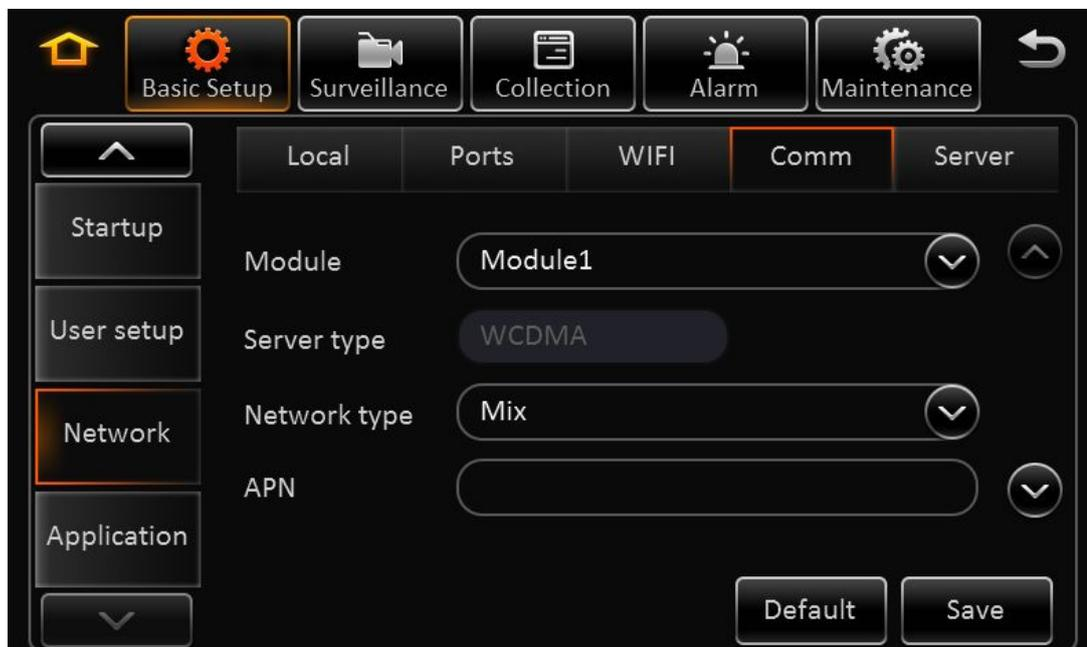
When entering the dialing setup interface, it searches the wireless module type automatically. It shows No Service when there is no module.
