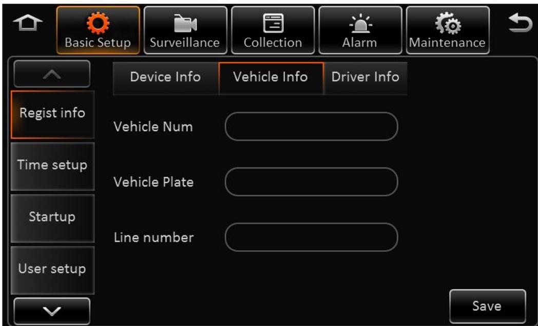
**Vehicle Number:** When connected with PAD, the vehicle number is needed.
