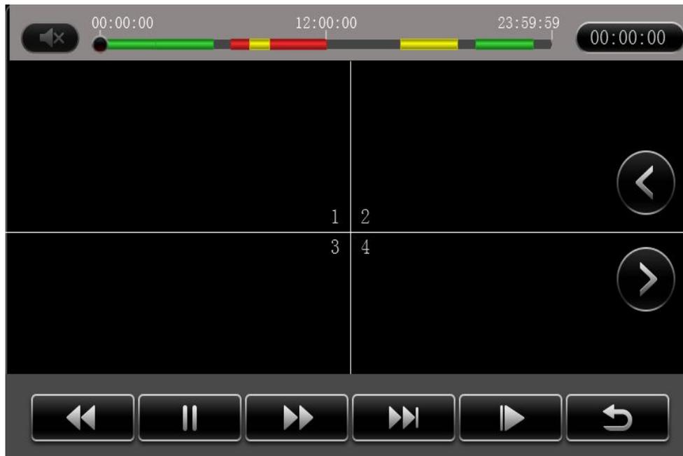
In playback interface, user can choose fast forward or fast backward to play the video, the button in the middle of screen can switch the channels. The image stops and it will not exit automatically when playing to the last video of the day.
