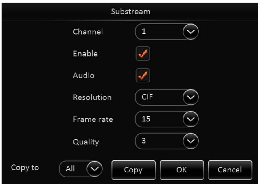
Sub stream includes channel number, enable or not, audio, resolution, frame rate and image quality.
