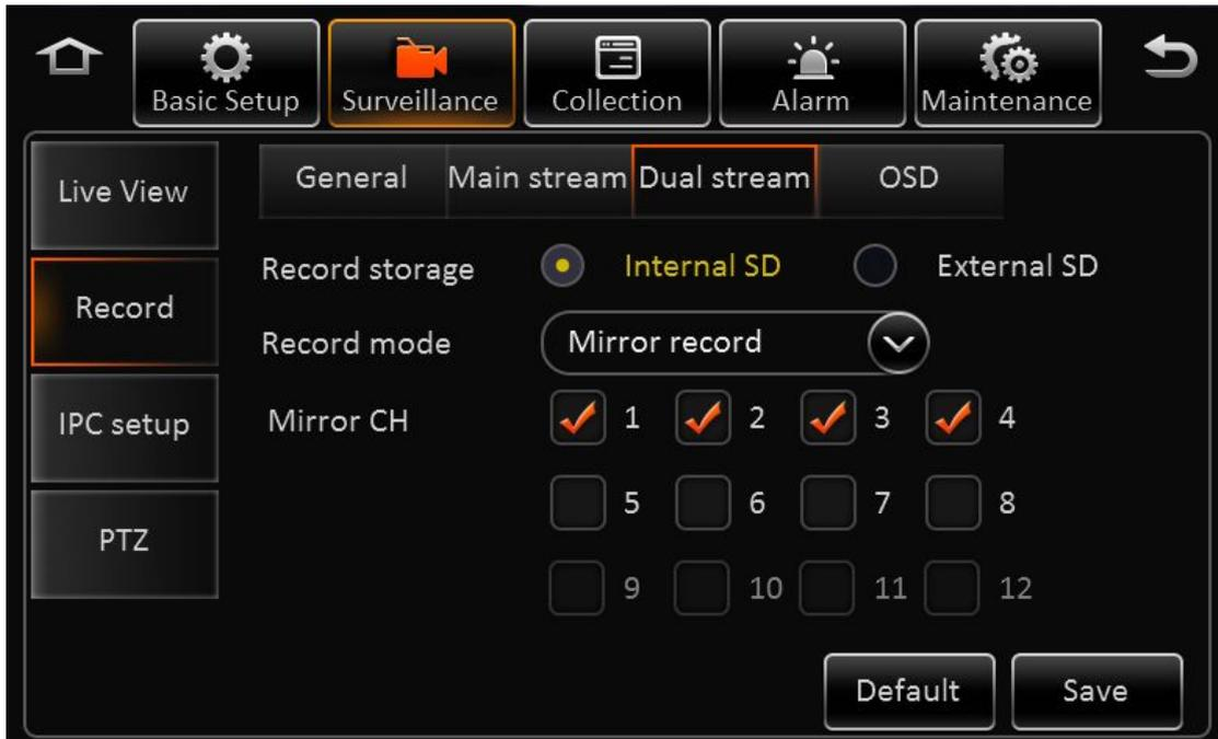
**Storage:** The storage type for sub stream, internal SD and external SD optional.
