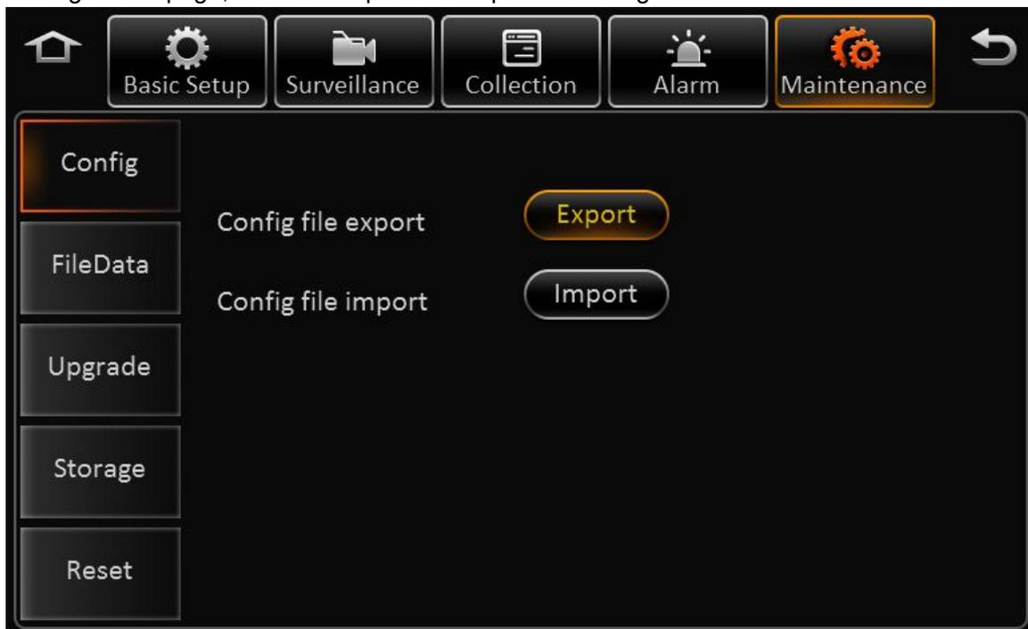
Insert flash drive to export the configuration file to the root folder, the file name is *ConfigFile*
