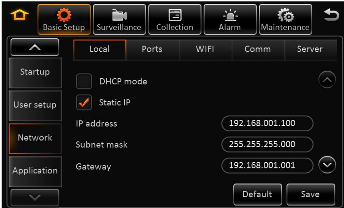
**Automatically obtain IP:** Dynamic acquisition, DNS can also be statically configured to dynamically obtain.
