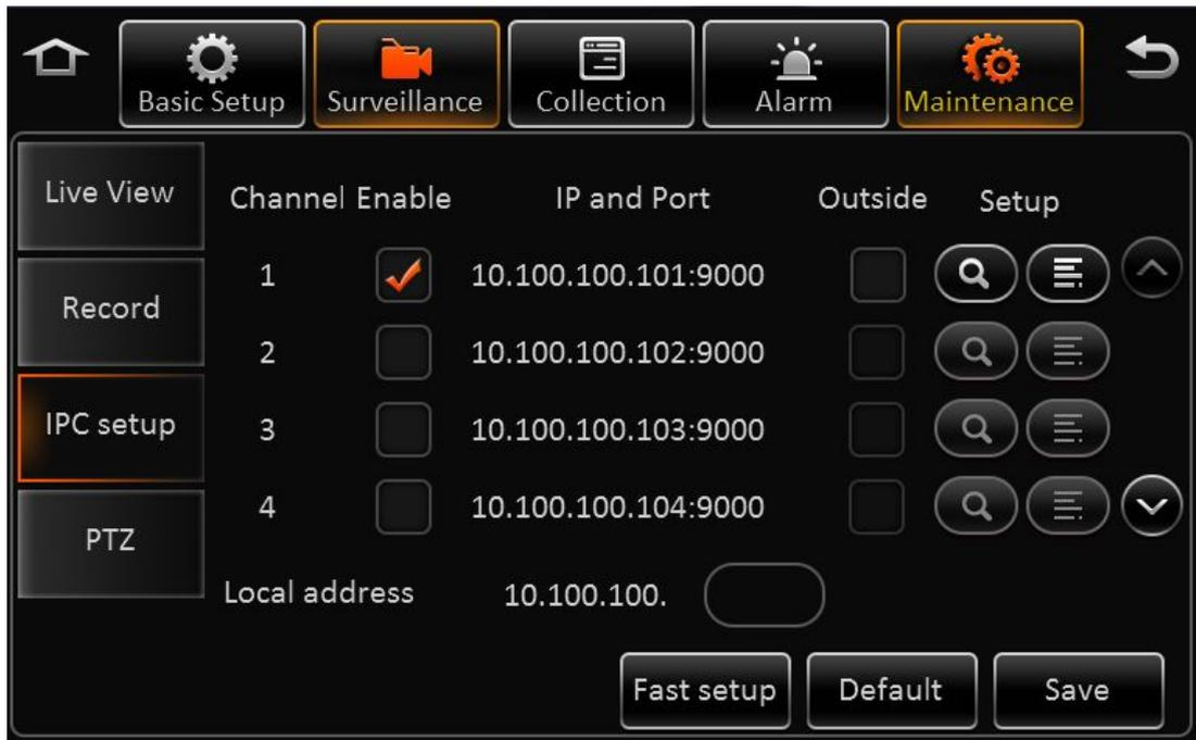
**Channel:** It includes the analog channels and IPC channels. Analog channel will not be shown if it connects to network camera.
