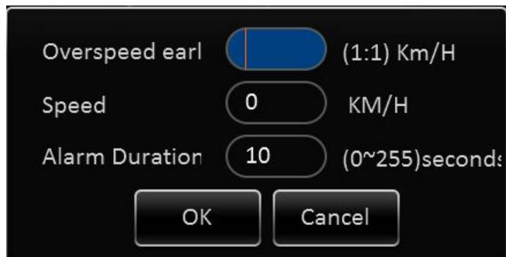
**Over speed pre alarm difference:** To set the pre alarm data. For example, if speed is 60 km/hour, and over speed pre alarm difference is 10 km/hour, TSS sends over speed alarm broadcast and records when it reaches 50 km/h.
