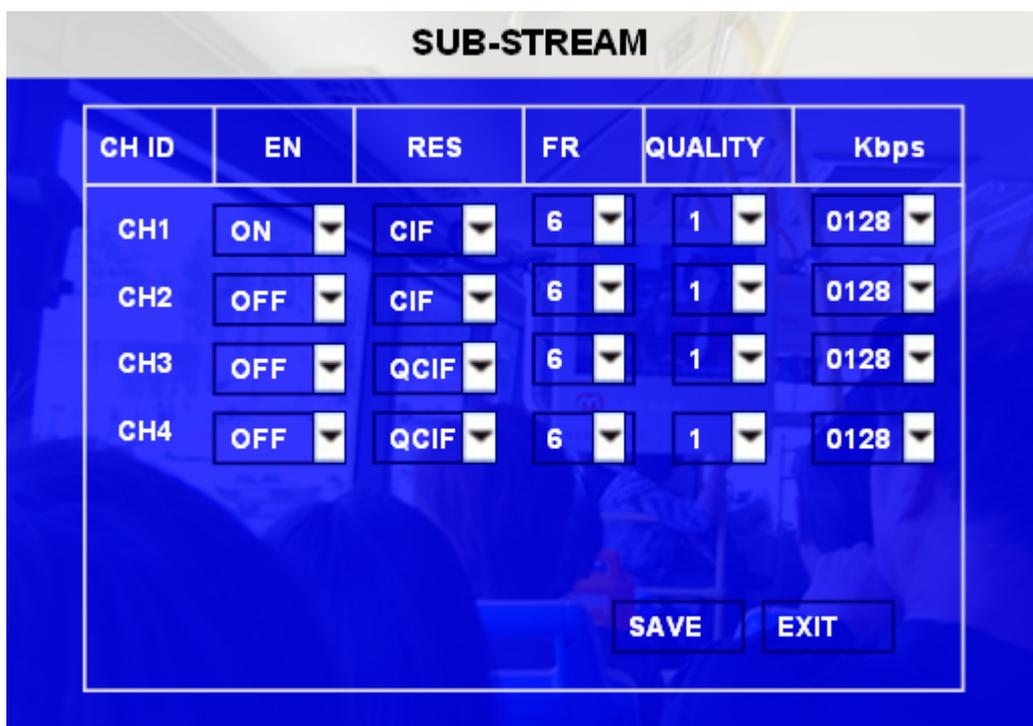
EN = enable the channels, required to be **ON** (make sure all channel sub-stream are on)
