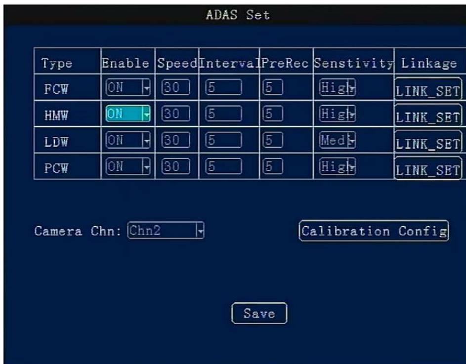
ADAS supports **FCW** (Forward Collision Warning), **HMW** (Headway Monitoring Warning), **LDW** (Lane Departure Warning), **PCW** (Pedestrian Collision Warning).
