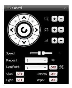
PTZ can be settled with 8 directions, Zoom, Focus, Lens, Distance, Preset Positions,
