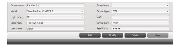
Editing equipment: selected equipment and then click the "Modify" button to change the relevant parameters, and then click the "save" button to save the new parameters.
