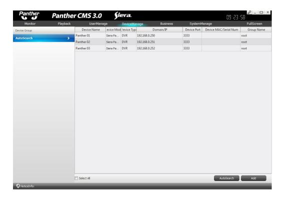
Click on "AutoSearch" button, wait a little, to be the equipment appears, check the need to add the device and click "add" buttons equipment will be added to the corresponding encoding or decoding device list, add support equipment.
